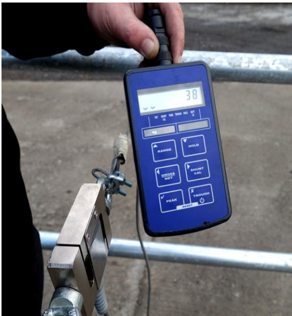
Test 1 Fh 1 top rail 38kg
